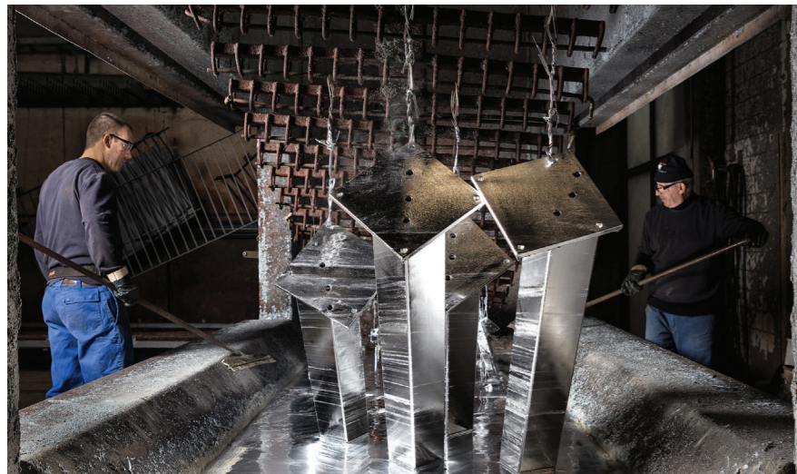
The combination of hot-dip galvanizing and powder coating using the duplex process ensures a particularly high level of corrosion protection.
