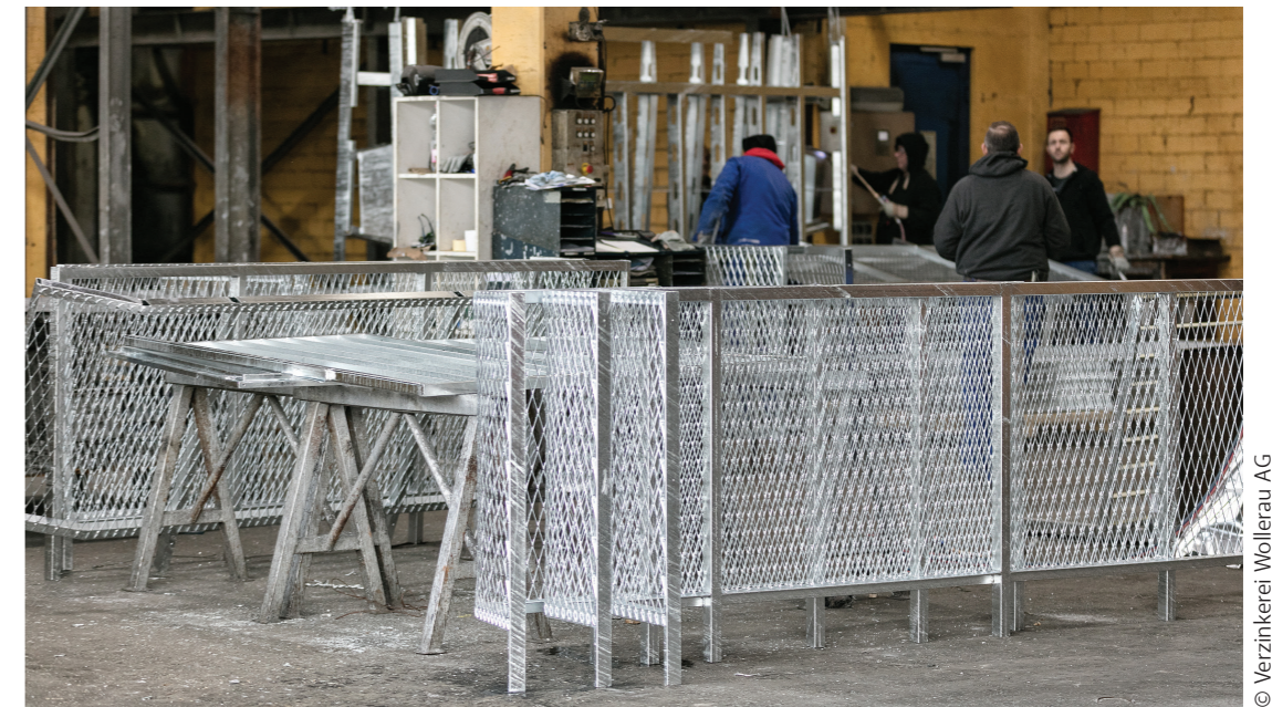
For higher corrosion protection requirements and design applications, the zinc coating is additionally protected by a powder coating.
